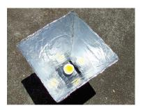
Now you are ready to cook. To help speed up the cooking process, you can add an isolative barrier between the food and the air. In this photo, we have placed an egg in a small cooking dish and covered the dish with plastic for insulation.
