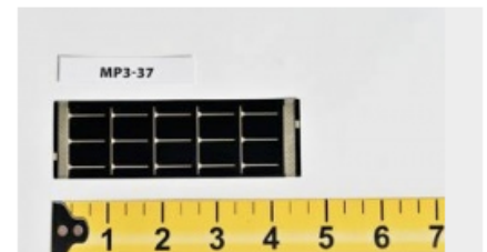
Operating Voltage: 3.0 Volts; Operating current: 50 milliAmps
